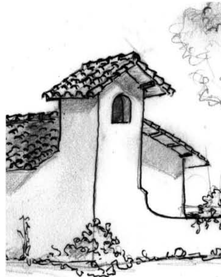
Because the rooftop water tank must be placed at the highest point on the roof, a tower can be integrated to contain this tank, becoming a distinctive architectural feature.
