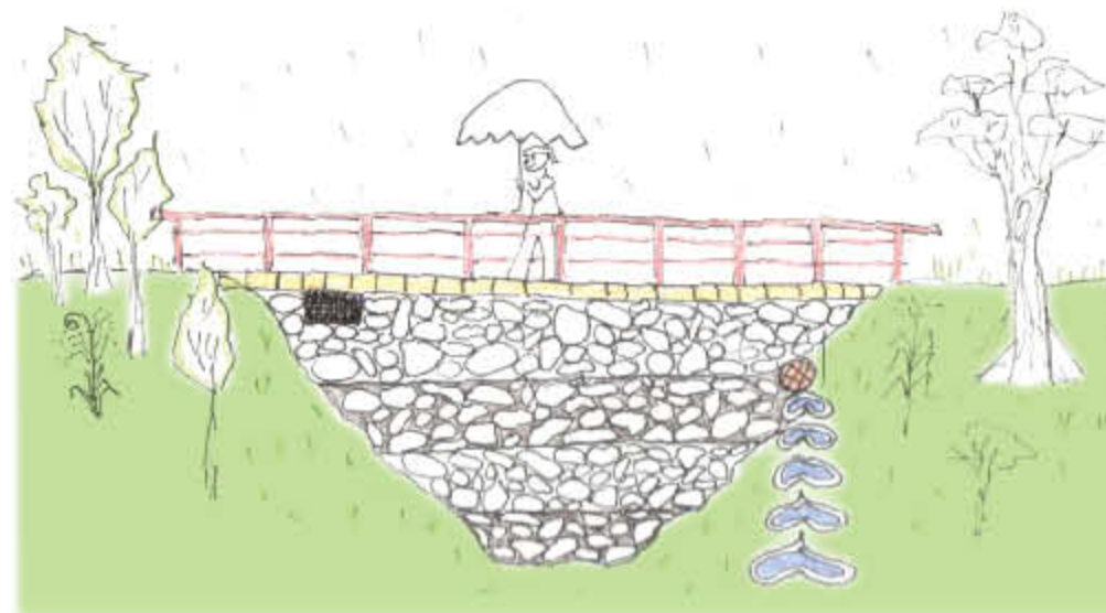
View of dam, gabion construction
